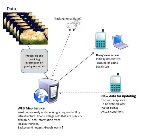
**Figure 1.** Basic concept on information flow from remote sensing data to grazing information to be accessible from computers and smart phones. Dashed lines illustrate features to be included later on.
